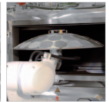
Dome transfer through dedicated side port
