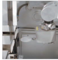
Precise handling of wafer by robot
